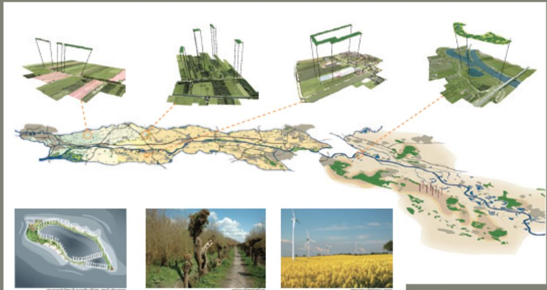
The plan contains 3 large interventions. The first one is an energyisland in the Northsea. This island contains 350 windmills and also has the ability to store energy by pumping water out of a big lake (off peak situation) and hydraulic produce energy by letting water in (high demand).
